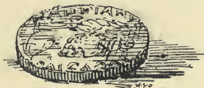
FLAN STAMPED FROM SHEET-METAL. FIG. 12.
